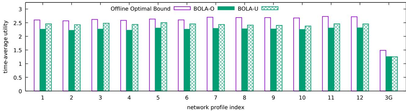
Fig. 9. The time-average utility of BOLA-O and BOLA-U with  $\gamma p = 5$  and a 25-second buffer playing a 30-minute video for the DASH test network profiles 1–12 and mobile traces (3G). BOLA utility is within 84–95% of offline optimal utility.
