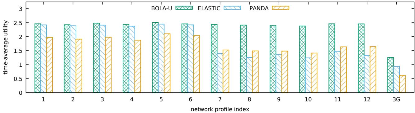
Fig. 11. The time-average utility of BOLA-U, ELASTIC and PANDA with  $\gamma p = 5$  playing a 30-minute video for the DASH test network profiles 1–12 and mobile traces (3G). Compared with ELASTIC and PANDA, BOLA-U has about 1.75 times the utility of the other algorithms in roughly half the cases.
